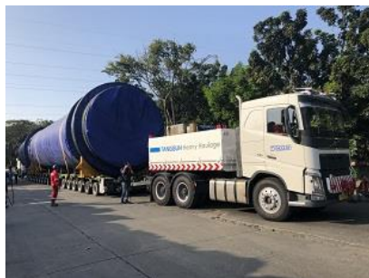
Multi Axle Trailer use for tank transportation
